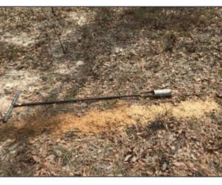
Soil Auger Next to Soil Core for Soil Unit Conformation
