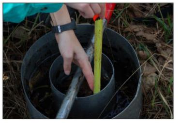
Measuring Water Level in Double-Ring Infiltrometer
