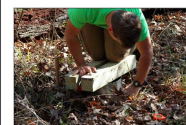
Making Sure the Infiltrometer is Properly in the Ground
