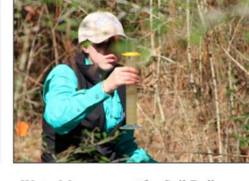
Water Measurement for Soil Bulk Density Hole
