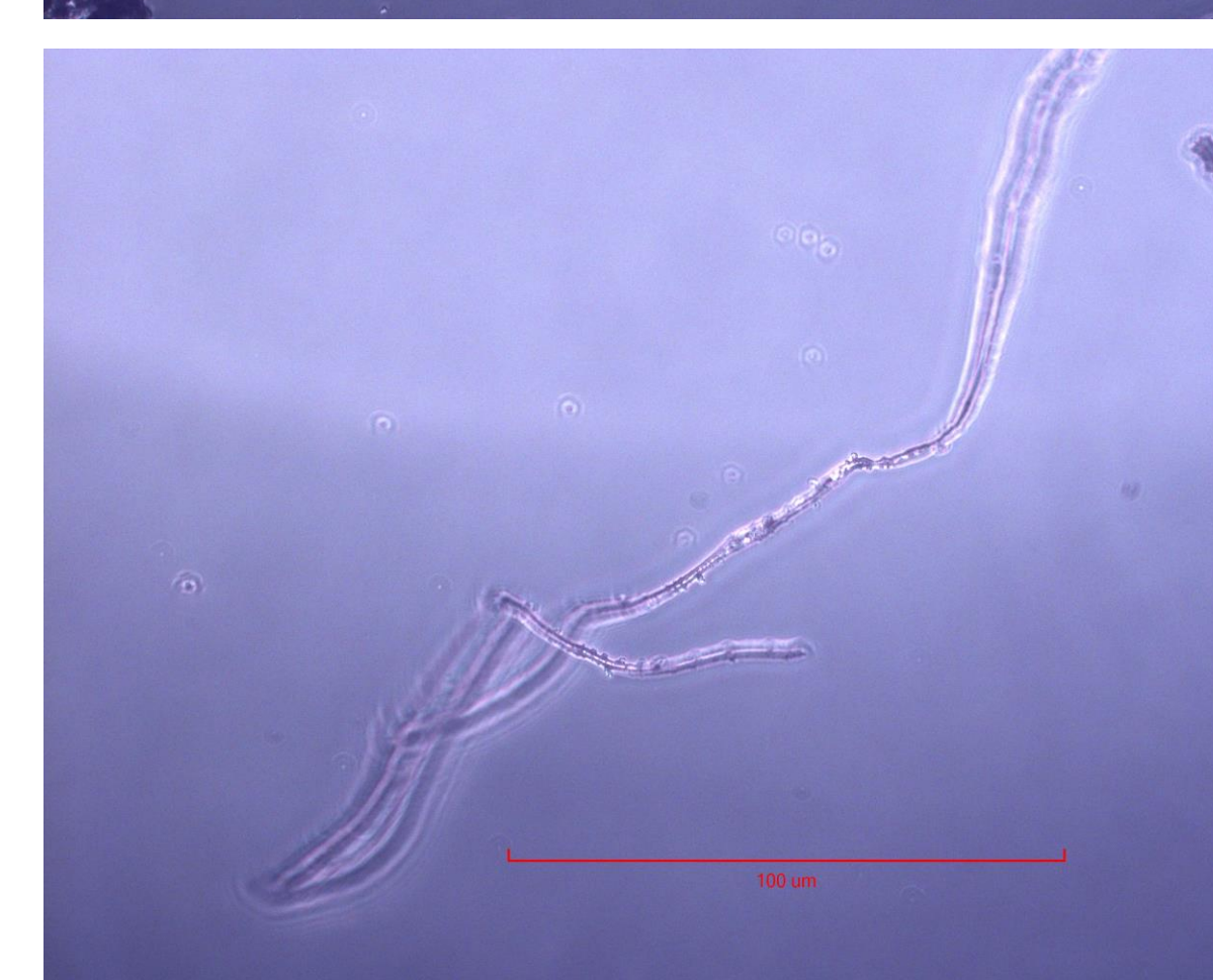
Figure 7: LWWTP biosolid sample: 150 μm < x < 850 μm filament
