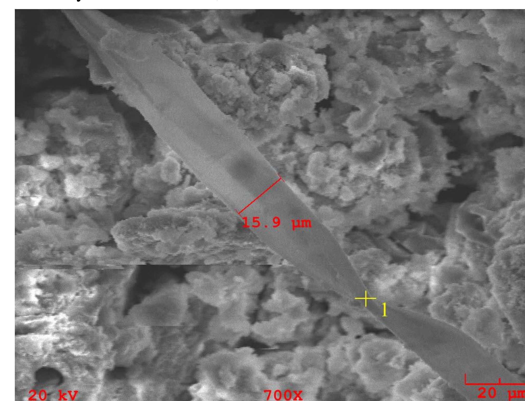
Figure 6 – SEM Micrograph Showing MP Filament
