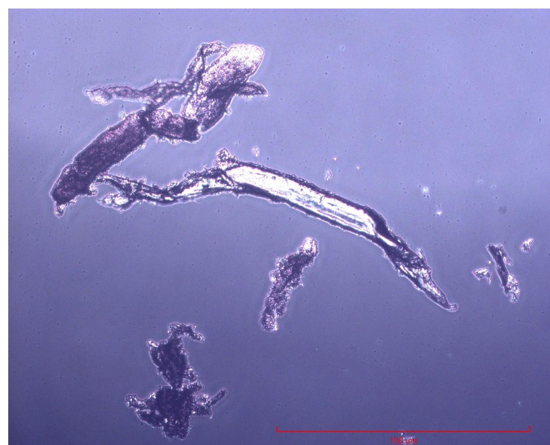
Figure 2 – Brightfield Microscopy Image of MP Fibers
