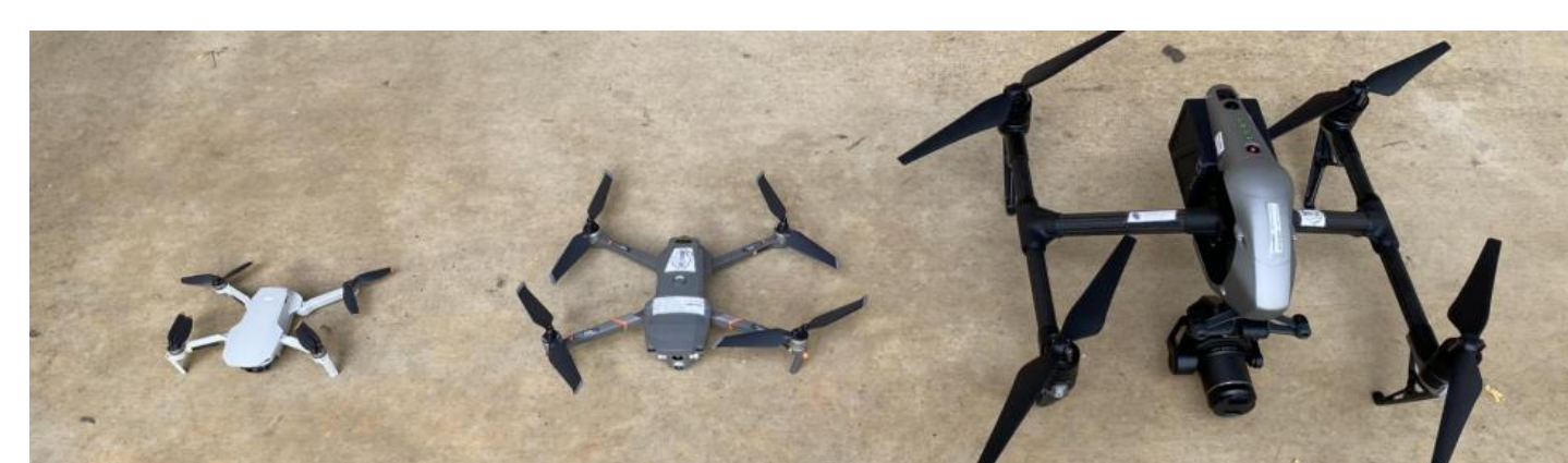
Figure 3: Three examples of drones tested: DJI Mini 2, DJI Mavic 2 Enterprise Advanced, DJI Inspire 2
