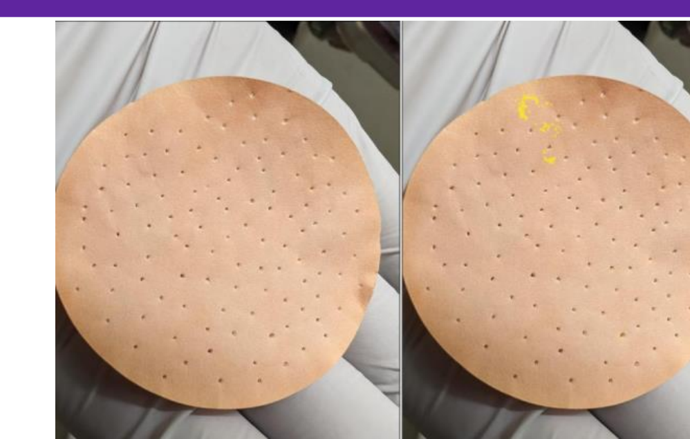
Figure 7: Photo of filter paper with mucus (left), false color mucus with image processing (right)
