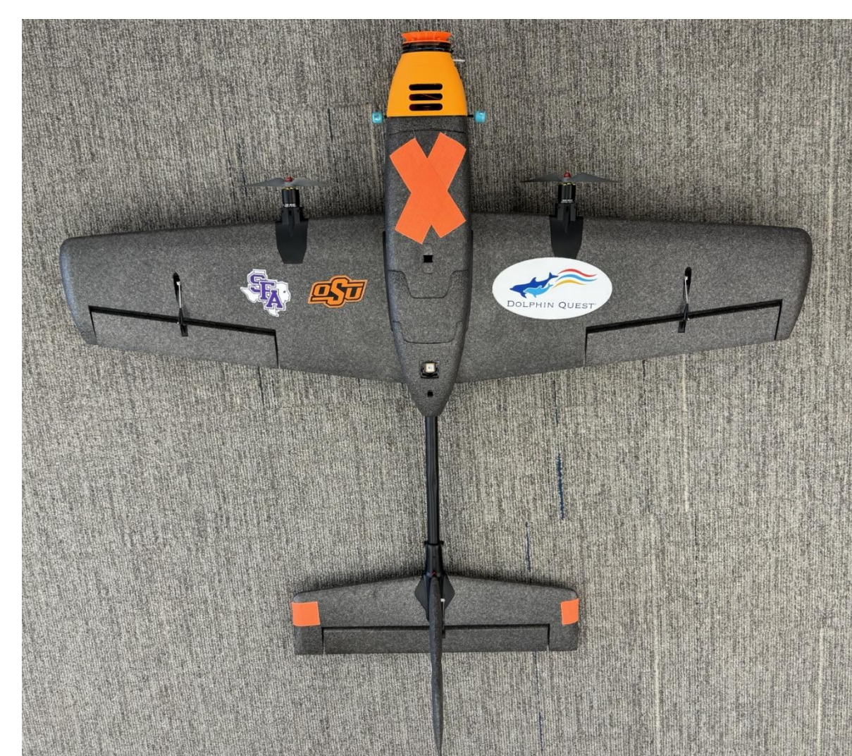
Figure 1: Modified Heewing T2 Cruza, PHASM prototype used in successful sample collection
